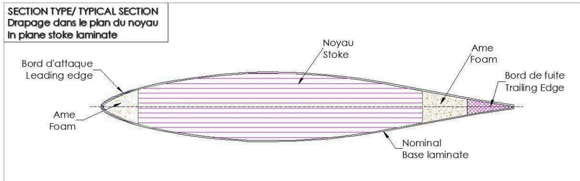
The structural core of the *foil* is manufactured (lay-up) as per the principle “parallel to the chord axis”; HM fibres are therefore permitted on the sole condition that these are laid up in strict compliance with the above drawing {parallel to the *foil* chord).
